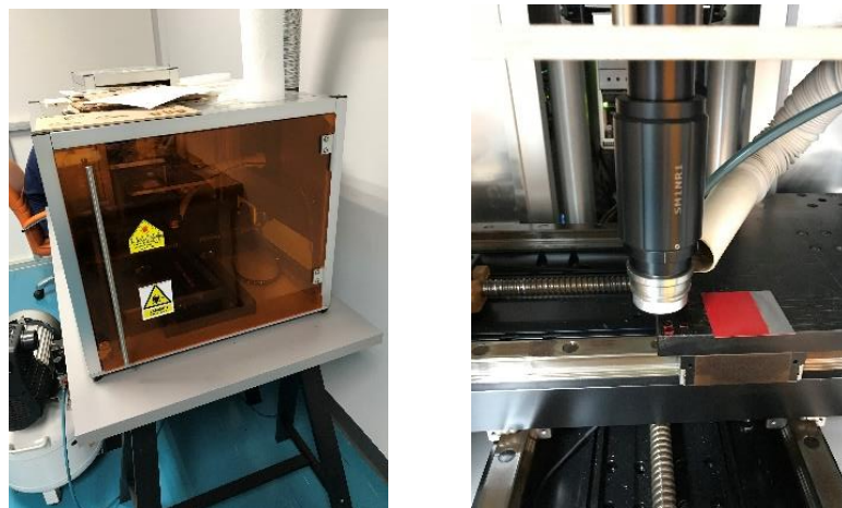
Figure 1: Experiment setup for graffiti removal using CO 2 laser
