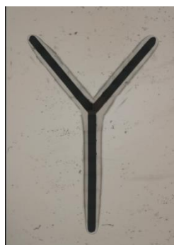
Figure 5: Microscope images (50X) of the microchannels obtained by laser writing of acrylic at laser fluences of 0.06 J/cm 2 for scanning speeds of 40 mm/s.
